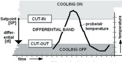
(cut out). For example: **SP** =10°C, **dI** =1.0°C: control between 9.0°C and 10°C. Another example: **SP** = 10°C, **dI** =3.0°C: control between 10°C and 13°C.
