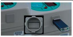
The USB plug provided can be left as is when logging is not required and no memory stick fitted. When logging is employed, cut 3 sides of the plug to allow a flap which raises for the memory stick as shown in the photo below.
